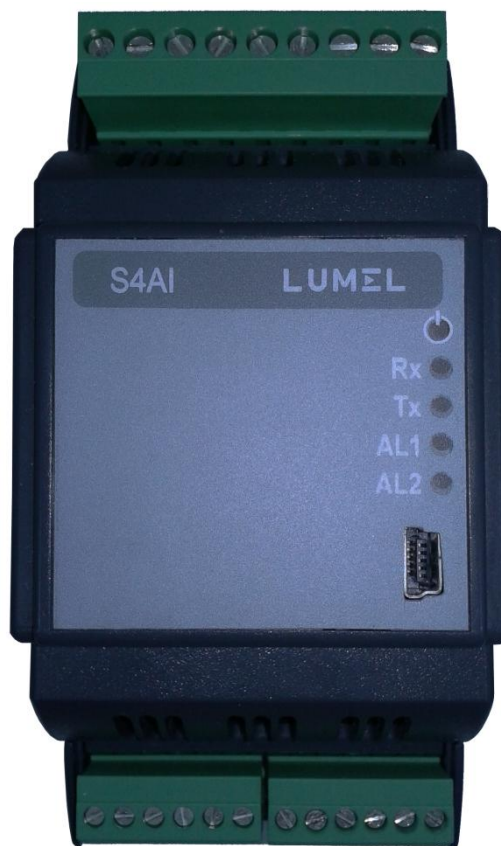
Fig. 1: View of S4AI module with detachable connectors
